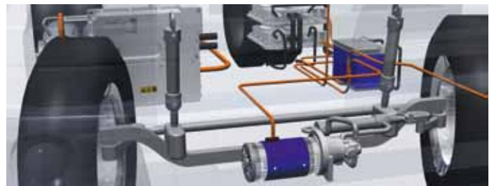
DCU: Demand controlled steering help pump
