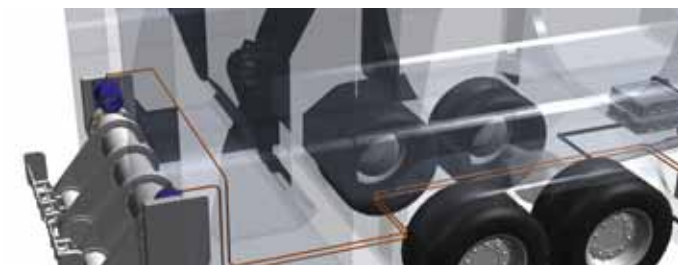
DCU: Lifting device – Position controlled system
