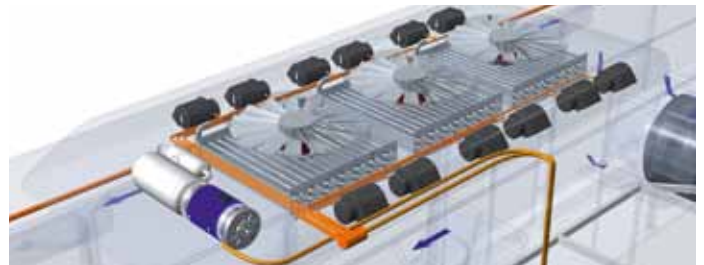
DCU/PSU: Controlling the compressor and the ventilation system
