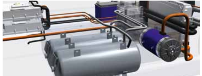
DCU: Demand controlled electric air compressor
